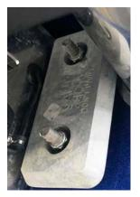
(oxidation) and metal reduction are the effects of operating in saltwater. To reduce these naturally occurring results on boat components, the sacrificial anodes attract and reduce most of the effects.
