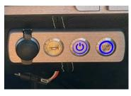
On a boat equipped with a Start-Stop button, press the button. If you are using the backup key, also turn the key to OFF. (Failing to do so means the electrical system will continue to function;
