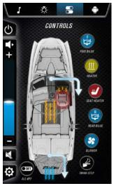
Touch the Forward Bilge to turn the forward bilge pump ON and OFF. If an Auto-Bilge Alert occurs, the driver will be able to navigate to the Controls page to see which bilge pump is running.
