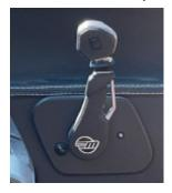
To the right of the boat operator is the shift/throttle lever. Any time the boat engine is off, the lever should be in the center upright position, which is Neutral (meaning the boat is not in gear) and is apparent when it can be felt slotting in with an auditory click. Boats are not equipped with "Park" like land-based vehicles.
