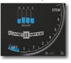
The Power Wedge is not intended for use at speeds greater than 26 mph. A notice will be displayed if the Power Wedge is in a deployed position at speeds exceeding 26 mph. Boat speed must be below 26 mph to dismiss the alarm. The Power Wedge
