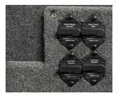
Power Wedge III, Surf Gate, and Stern Turn (if equipped) breakers are located on the board in the port rear closeout adjacent to the engine compartment. If any of these systems will not operate, verify that the supplemental breakers located in the port rear storage compartment are properly set.
