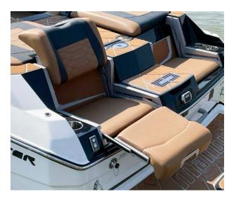
No one should sit or ride on the sun pads when the boat engine is running. Carbon monoxide is emitted from the exhaust system and vented into the water beneath the swim board. Fumes can and do reach the sun pad area. Avoidance of carbon monoxide poisoning is addressed in the *Safety* section of this manual.
