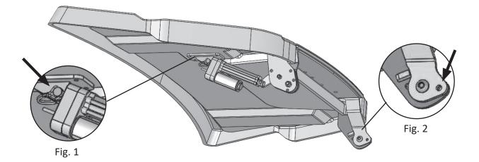
step is operational. When the button is released then the power step is locked out. However, the power step can still be deployed manually (see *In Case of Emergency* below) while in locked out mode. When transporting your boat, the powered swim step should be in the stowed position.
