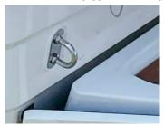
apex of the hull under the bow, and two transom eyes, which are located one each on the port and starboard sides of the transom. Thee semi-circular or U-shaped metal
