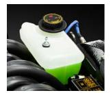
percent extended warranty antifreeze plus 50 percent distilled water. (Do not use tap or other water as other elements in the water can cause build ups or deposits within the closed cooling system. This can interfere with proper operation and resulting damage is not covered under warranty.)
