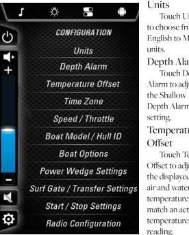
Touch Units to choose from English to Metric units. Depth Alarm Touch Depth Alarm to adjust the Shallow Depth Alarm setting. Temperature Offset Touch Temp Offset to adjust the displayed air and water temperatures to match an actual
