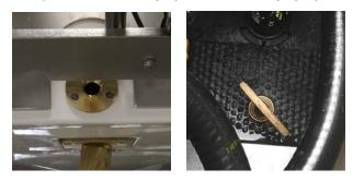
All boats are equipped with two drain plugs, a  $\frac{1}{2}$ " drain plug on the transom and a T-handle drain plug in the center of the boat. The  $\frac{1}{2}$ " drain plug can be accessed outside the boat, directly under the swim platform on the enter back of the transom. The T-handle can be accessed inside the boat through the center access. Be certain to read the above information regarding securely installing drain plugs prior to all outings.
