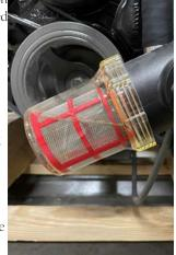
*and Maintenance* section in this manual for information on how to properly remove debris from the raw-water intake/ sea strainer.
